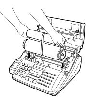
**5** Cut the band which holds the spools together with scissors, and remove it. Insert the remaining gear into the right end of the empty spool and the flange into the left end of the empty spool. Make sure the tabs on the gear and the flange fit into the slots in the ends of the spool (the gear has two tabs and the flange has one tab).
